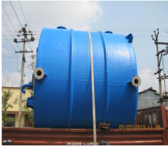
FRP Water Storage Tanks
