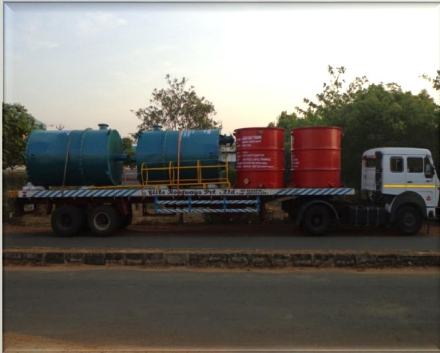
FRP Storage Tanks
